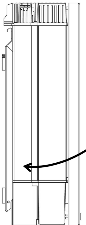
Illustration 6.5: Anbring inverteren i monteringsbeslaget
